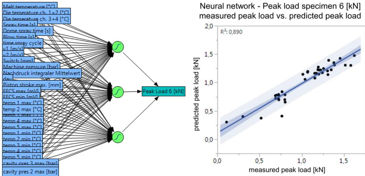
Figure 4: Model of neural network (left) and predicted peak load vs. measured values for neural networks (right) [6]
