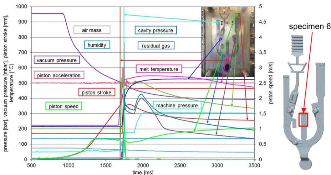
Figure 2: Shot curve with additional sensor signals
