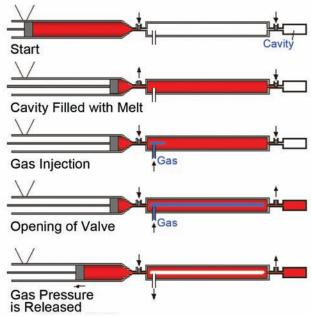
Figure 1 – Gas injection using a side cavity<sup>4</sup>.
