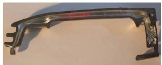
Figure 7 – Die casting produced by gas injection<sup>6,7</sup>.
