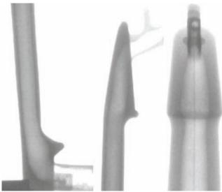
Figure 8 – X-ray of gas injected parts.
