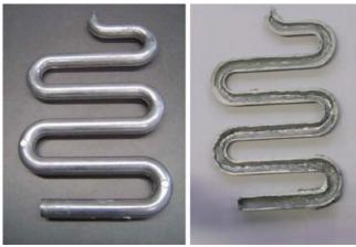
Figure 11 – Two casting geometries produced with gas injection.
