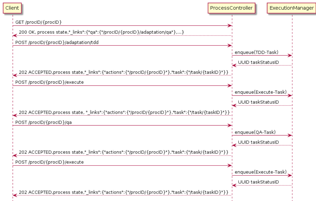
Figure 8. REST Client Server Interaction
