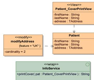
Figure 3.5. Entity Model Subset showing Adapter and View
